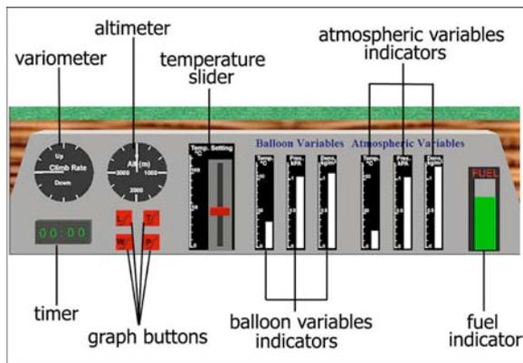
Figure 2: The control panel of a hot air balloon
